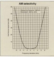
In this tuner, we have succeeded in achieving both low distortion and wide selectivity by using three very carefully manufactured and selected 4-element ceramic filters which have very flat group-delay characteristics. Without resorting to IF band switching, we've attained a very high selectivity of 85 dB ( $\pm400\,\mathrm{kHz}$ ), while distortion is a very low 0.1% (mono), 0.15% (stereo).
