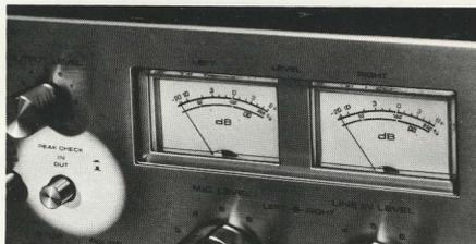
The dual VU meters may be switched from normal meter operation to a peak-reading mode to provide readings of high level signals that might be too brief to be detected by normal meter operation but could still result in distortion. The needles revert slowly so that the peaks will not be overlooked, to enable appropriate level compensation as needed.
